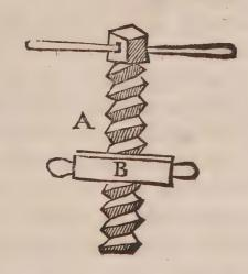
The former is noted in the figure with the letter A, the other with F. Aristotle himself doth not so much as mention this instrument, which yet notwithstanding is of greater force and subtilty, then any of the rest. It is chiefly applied to the squeezing or pressing of things downe-wards.
